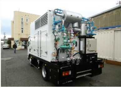
中圧減圧車 Medium pressure decompression vehicle
