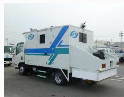
地中探査車 Underground exploration vehicle
